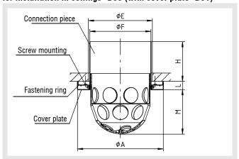
for installation in round ducts, -RAO/-RBO/-RCO (with curved blade -RA1/-RB1/-RC1)
