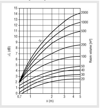
For  $V_R,$  the following values must be used: sound-attenuated room =  $V_R \ x \ 2,$  normal room =  $V_R \ and$  hard room =  $V_R \ x \ 0.5$
