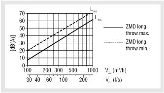
The values apply to hose connections. They decrease by approximately 4 dB for pressure duct connections.
