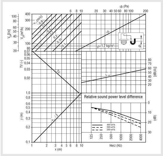
Read temperature ratio TV for determining the temperature  $\Delta T_x$  in the diagram. For the jet throw x + jet throw y, the value x from the diagram must be used.
