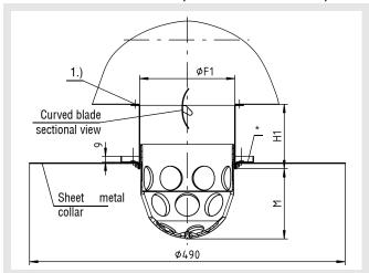
\*Fastening ring fitted only if delivered with sheet metal collar 1.) On-site mounting holes
