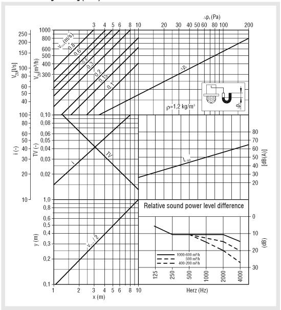
Read temperature ratio TV for determining the temperature  $\Delta T_x$  in the diagram. For the jet throw x + jet throw y, the value x from the diagram must be used.
