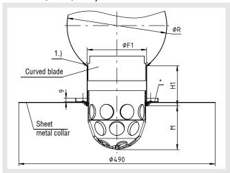
\*Fastening ring fitted only if delivered with sheet metal collar 1.) Mounting holes without curved blade
