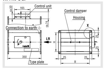
The VM-PRO-Q-Ex is delivered in right-hand design only. If the layout of the control unit is required on the left side, then VM-PRO-Q-Ex must be rotated by 180°.
