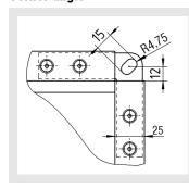
As standard, the volumetric flow controller VM-PRO-Q-Ex is delivered with corner angle. The special form of the corner holes allows them to be connected to the connection systems available on the market (e.g. Metu system M 2/M 3)
