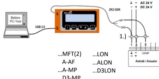
Local connection via a connecting cable of the MF/MP or LON drive using a ZK2-GEN cable.
