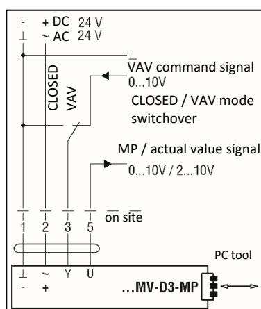
MP bus activation with integrated switch-
