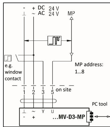
**Lock mode (CLOSED):** In the 2...10 V mode, the following function can be carried out with a 0 - 10 V signal.
