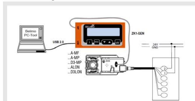
Local connection via a service socket of the MF/MP or LON drive using a ZK1-GEN cable.
