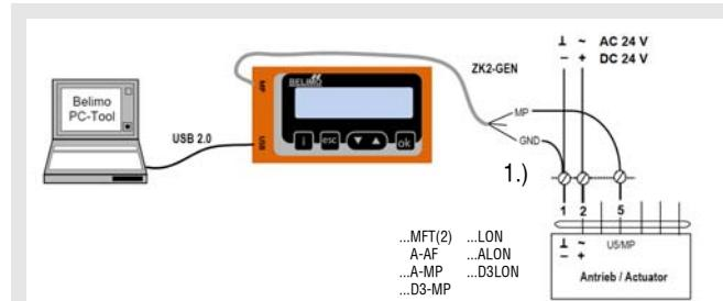
Local connection via a connecting cable of the MF/MP or LON drive using a ZK2-GEN cable.
