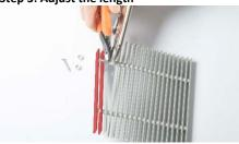
• Cut off the protruding part of the spring.
