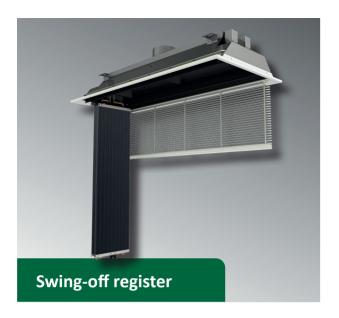
The register swinging down without tools is recommended particularly for applications in hospitals or rooms, for instance, in which high requirements pursuant to VDI6022 are imposed. For the register can be swung out without having to disconnect the hydraulic circuit, thus ensures simple cleaning from all sides and provides access to the interior parts which are in contact with secondary air.
