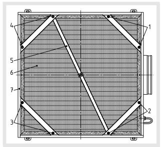
With built-in spacers for fixing the filter clamps.
