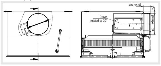
Attention! With the FKU-V model, the actuator cannot be mounted to the shut-off damper!
