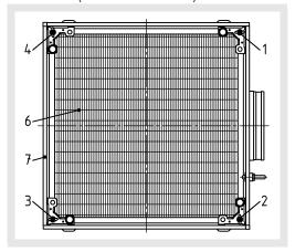
Diffusers with pole brace fastening (-VM) NW 400-800
