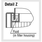
Loosen filter clamp (pos. 4) and remove it along with shipping brace. Press the particle filter unit (pos. 6) with the fluid seal (see detail Z) pointing upwards into the filter housing (pos. 7). Take care that the filter material is not irreparably damaged. The filter unit can be easily locked us-
