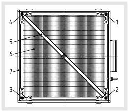
With built-in spacers for fixing the filter clamps.
