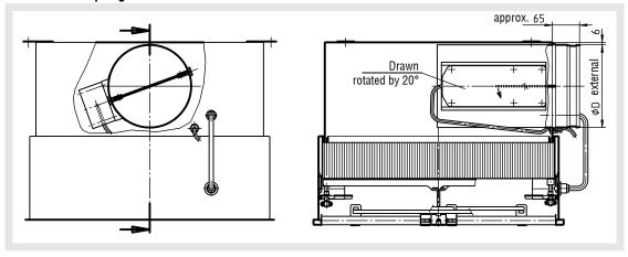
Attention! With the FKF-V model, the actuator cannot be mounted to the shut-off damper!
