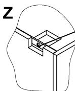
External insulation (-la) recessed in the area of the mounting brackets.
