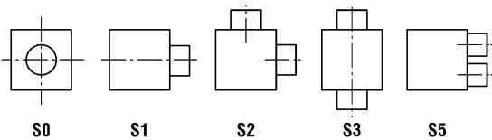
Minimum height [KHS] with spigot position S1+S2+S3+S5 = spigot diameter øD +137 mm and with spigot position S0 = 235 mm.
