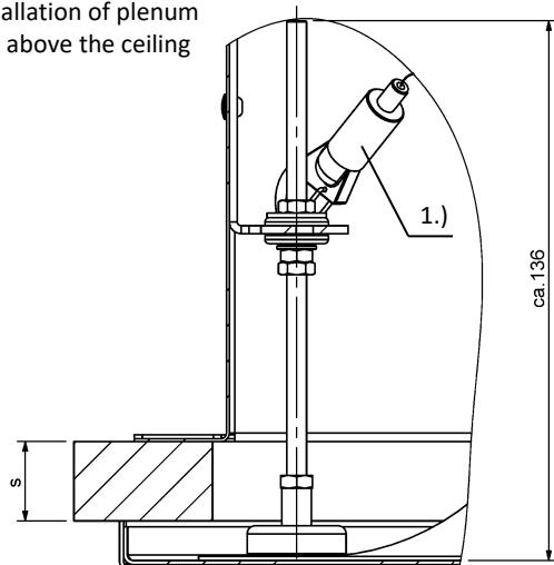
Installation of plenum box under the ceiling
