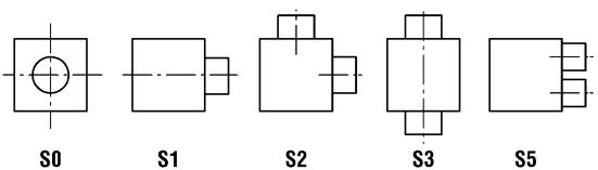
Minimum height [KHS] with spigot position S1+S2+S3+S5 = spigot diameter ØD + 102 mm and with spigot position S0 = 200 mm.
