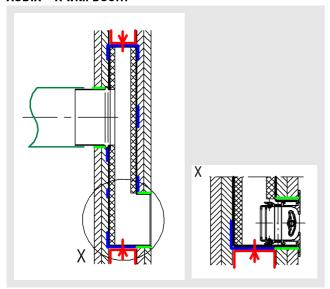
Flexible air duct connection additional on-site sound-absorbing strips, if necessary C wall profile
