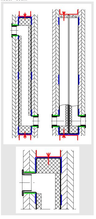
Additional on-site sound-absorbing strips C wall profile
